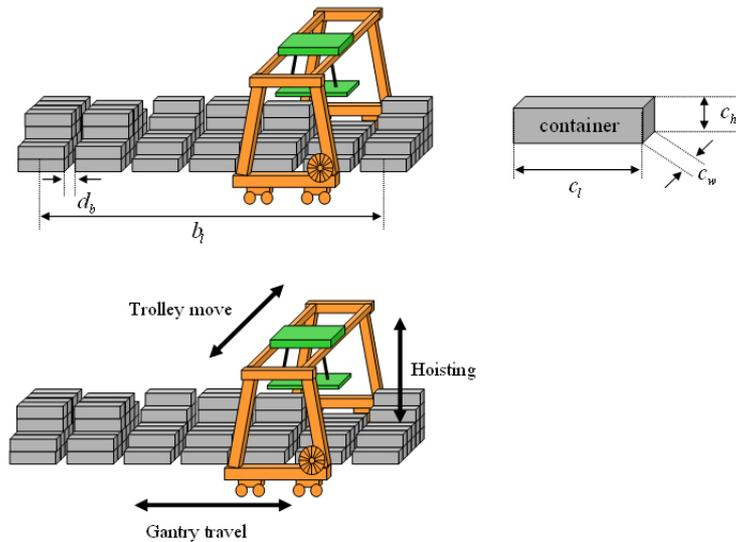
**Figure 3.** Illustrations of notations and terminologies on blocks
