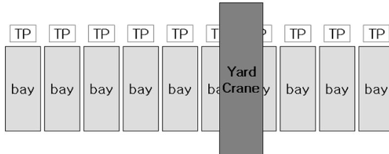
**Figure 1.** A block with TPs at a side of each bay
